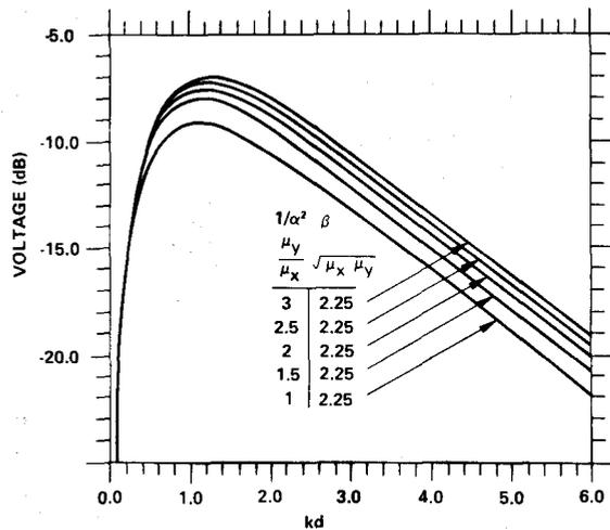
Fig. 4. Voltage response level (dB) versus normalized wavenumber  $kd$  for unbiased recording.  $k = 2\pi/\lambda$ ,  $\lambda$  is the wavelength,  $d$  is the depth of recording.  $\beta = 2.25$  is a typical mean permeability.
