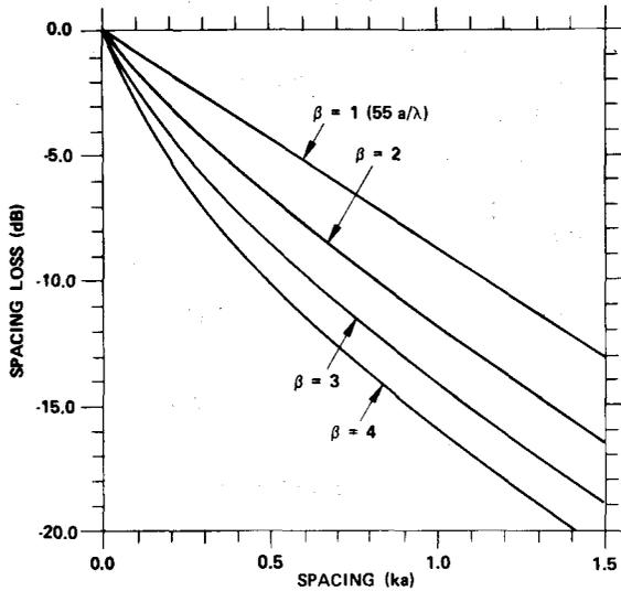
Fig. 2. Effect of head-to-medium spacing on the reproduce flux. Spacing loss (dB) is plotted versus normalized spacing  $ka$  where  $k = 2\pi/\lambda$ ;  $\lambda$  is the wavelength and  $a$  is head-to-medium spacing.  $\beta$  is the mean geometric permeability.
