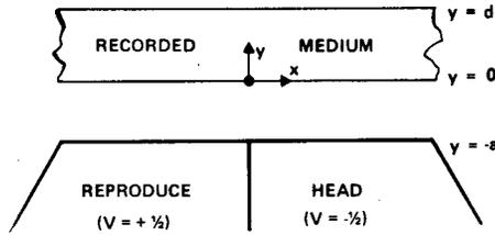
Fig. 1. Two-dimensional geometry for the reproduce flux calculation.  $d$  represents the depth of recording which may be less than the coating thickness. Boundary potentials on the head surface are indicated for derivation of field per unit MMF.
