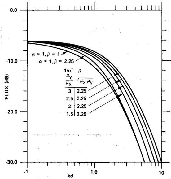
Fig. 3. Flux response level (dB) versus normalized wavenumber  $kd$  for ac biased recording.  $\beta = 2.25$  represents a mean permeability typical for many recording materials.
