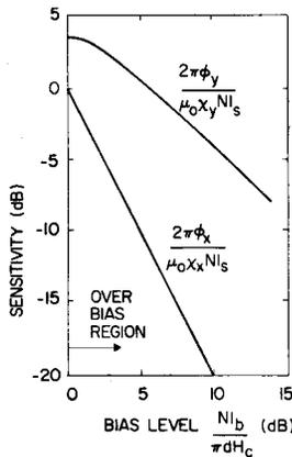
Fig. 10. Tape flux vs. bias due to longitudinally (x) and vertically (y) recorded magnetization components by a zero gap length record head. 0 dB bias denotes maximum sensitivity from recording through to the back of the tape coating.
