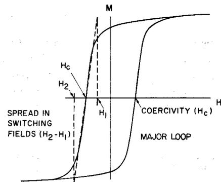
Fig. 4. Major loop of typical tape material.
