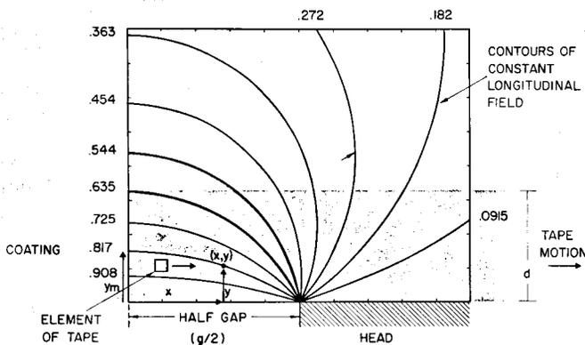
Fig. 6. Contours of constant longitudinal field in region above recording head surface. Left-hand edge is gap centerline. Contour magnitudes are in fraction of deep gap field. Tape magnetic coating is shaded with a typical element of tape demarked for text discussion of magnetizing process.
