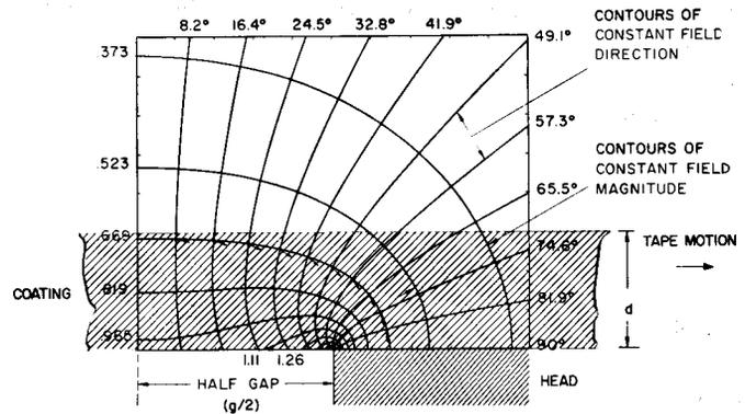
Fig. 11. Contours of constant total field and field direction. Head is same as in Fig. 6 except here field direction contours are shown where angle is deviation down from horizontal (explicitly shown on contour 0.669).
