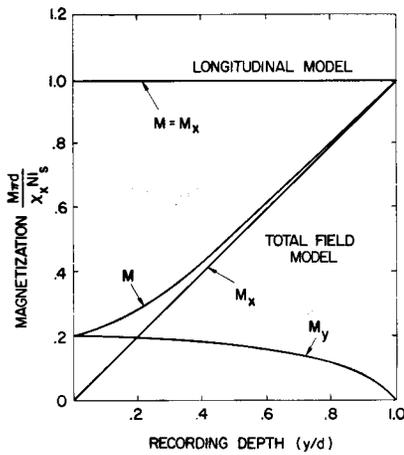
Fig. 9. Recorded magnetization vs. depth into tape for longitudinal and total field models. The bias has been set to record through to the back of the coating. The zero gap length limit is considered for both models.
