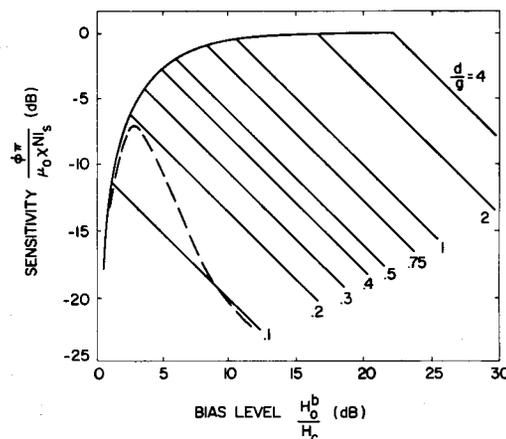
Fig. 7. Output vs. bias for various coating thickness to gap ratios ( $d/g$ ) using longitudinal model. Dashed line is data for a  $\gamma\text{Fe}_2\text{O}_3$  tape placed to match peak output point.
