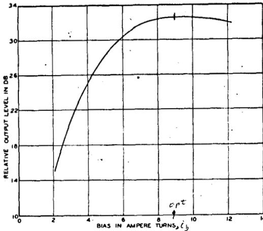
Fig. 8—Output-level-versus-bias, Minnesota Mining black-oxide plastic tape.
