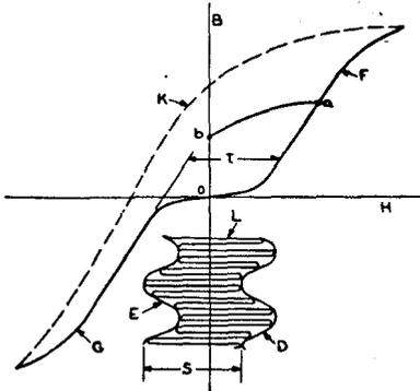
Fig. 1—Diagram showing how virgin-tape characteristic is modulated.
