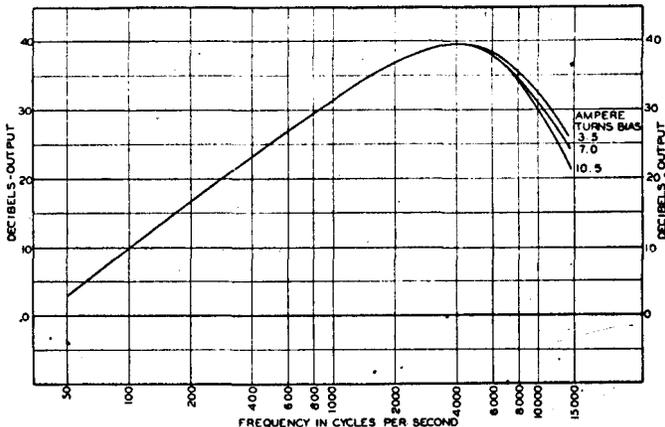
Fig. 13—Frequency response, Minnesota Mining Type RR tape.
