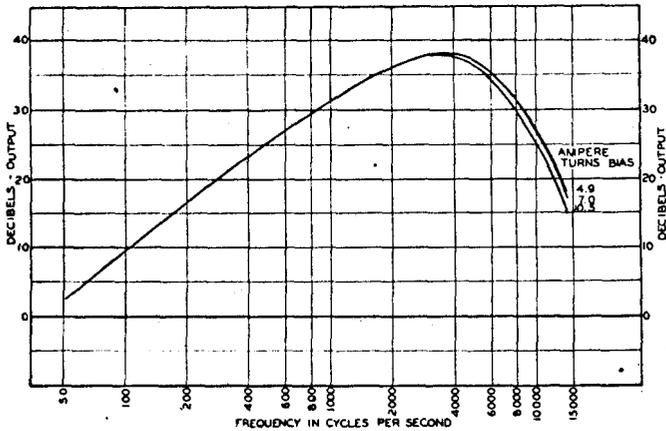
Fig. 12—Frequency response, Minnesota Mining black-oxide plastic tape.
