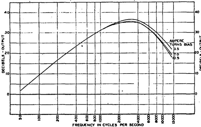
Fig. 11—Frequency response, duPont SW4 tape.
