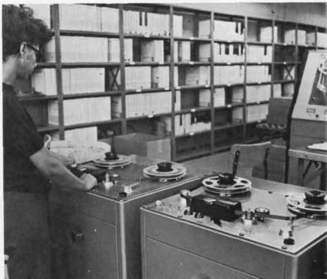
Fig. 2. This line of ten cassette duplicators can produce as many as 10,000 albums a day if it is operated on an around-the-clock basis.
