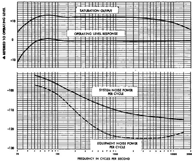
FIG. 2. Plot of 30 ips saturation, response, and noise density as a function of frequency. (Full track, 3 M 203 tape. Data taken on an Ampex MR-70 tape recorder using 17.5  $\mu$ sec post-emphasis and no low-frequency pre-emphasis, 150 kc bias, and a 234 mil wide reproduce head with 180  $\mu$ in. gap.)
