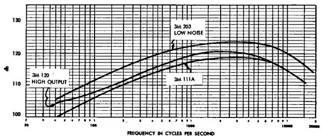
FIG. 6. Dynamic range as a function of frequency for three styles of tape. (15 ips, full track.)
