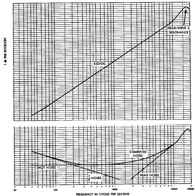
FIG. 8. Signal and noise as a function of frequency from a conventional reproducing head-preamplifier system. (Hypothetical case. All equalization removed.)
