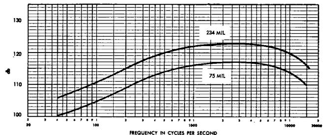
FIG. 5. Dynamic range as a function of frequency for track widths of 75 and 234 mil. (15 ips, 3M 203 tape.)
