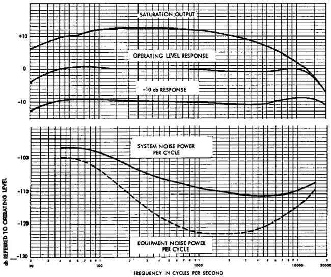
FIG. 3. Plot of 7½ ips saturation, response, and noise density as a function of frequency. (Full track, 3M 203 tape. Data taken on an Ampex MR-70 tape recorder using NAB equalization, 150 kc bias, and a 234 mil wide reproduce head with 180  $\mu$ in. gap.)
