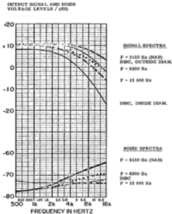
**Fig. 2** Saturation signal and 1/3-octave noise spectra. Heavy curves: For a fourth-generation master tape with various reproducing transition frequencies F = 3150 Hz (NAB), 6300 Hz, and 12 500 Hz. Light curves: For a 33 1/3 rev/min vinyl disk pressing. See footnotes 3 and 4 for detailed conditions.
