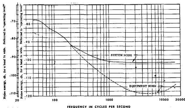
Fig. 1—Noise spectrum analysis. HP 302A wave analyzer, 7-c stand-bandwidth. Ampex Model 351, one-quarter inch full-track, 15-ips, NAB equalization. Irish 211 tape, biased to "peak" at 15-mil recorded wavelength.
