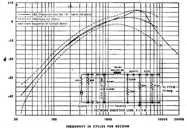
Fig. 5—Response-frequency characteristics and circuit of network for objective noise measurement.
