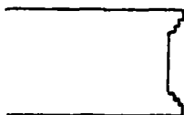
Fig. 8. Cross-section of a worn head face, showing stepped pattern of the wear which lifts the tape out of intimate contact with the head face.
