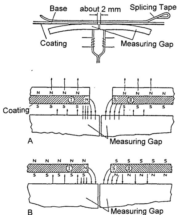
Fig. 2. Method for determining the perpendicular component of the dc magnetization.
