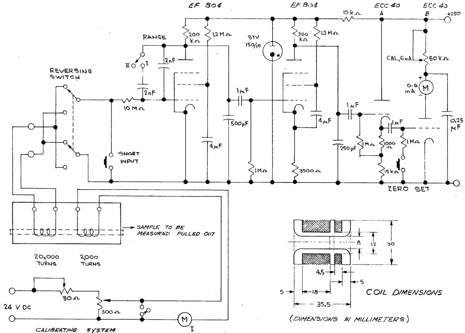
Fig. 5. Schematic diagram of electronic fluxmeter, circuit for calibrating it, and construction of induction coil.
